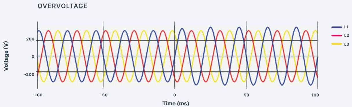
Figure 7 Overvoltage - The voltage slightly rises on line L1, surpassing the regulatory threshold.
