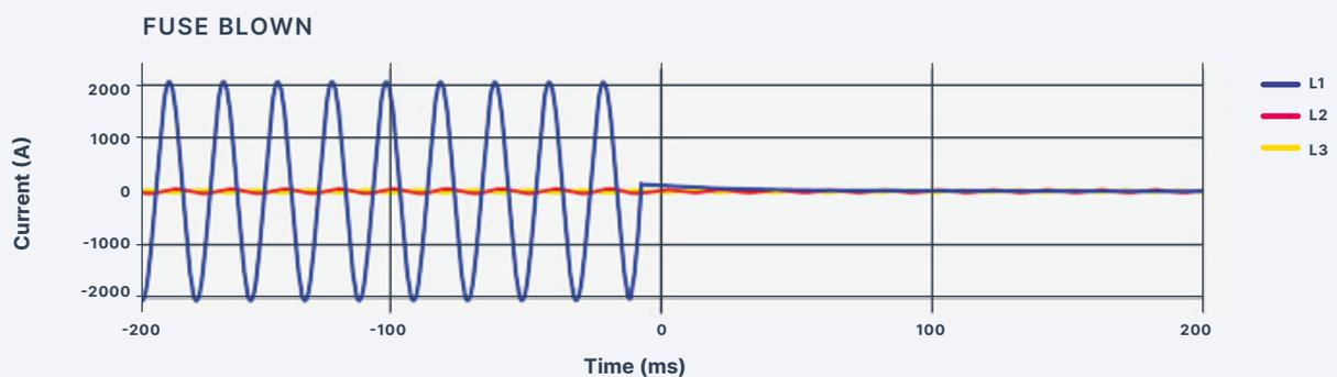
Figure 5 Fuse Blown - Current waveform associated with a fuse blowing and clearing a line-to-ground short-circuit fault.
