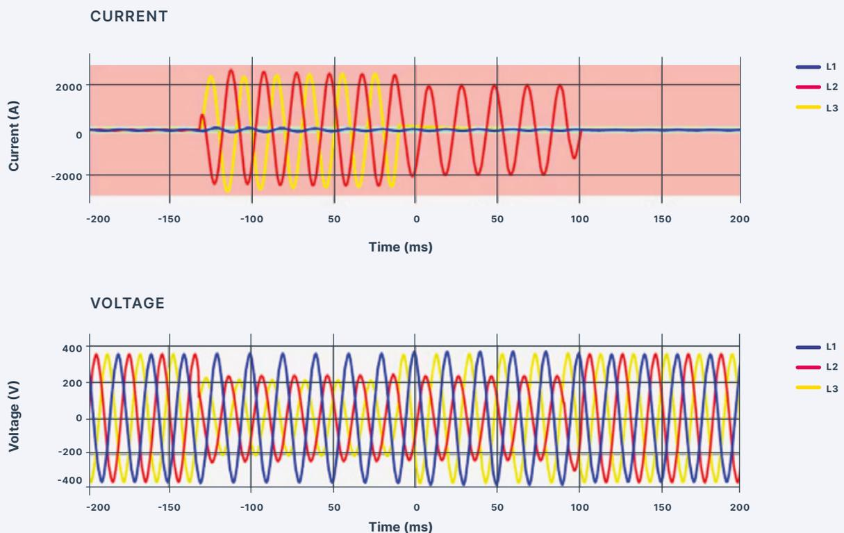
Figure 9 Waveform Capture for Short-Circuit event.
