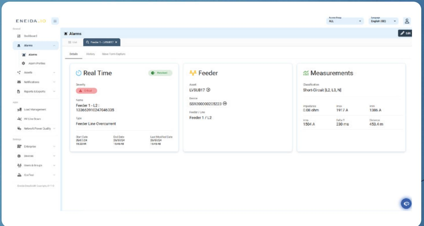
Figure 10 Impedance and Distance to Fault in Alarm Details page for a Short-Circuit event.
