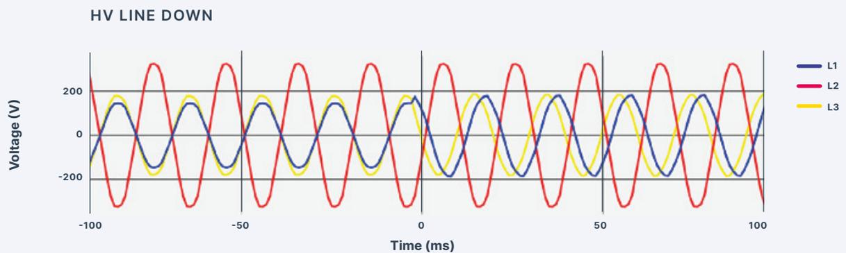
Figure 8 HV Line Down - Moment when an HV overhead line breaks, interrupting the voltage supply on one phase of the HV network and impacting the voltages on the LV side.
