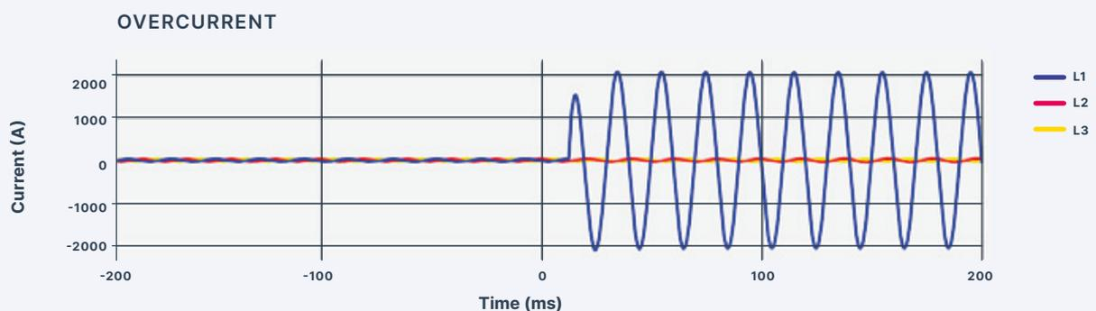
Figure 4 Overcurrent - Ignition of a line-to-ground short-circuit fault, detected by an overcurrent alarm.
