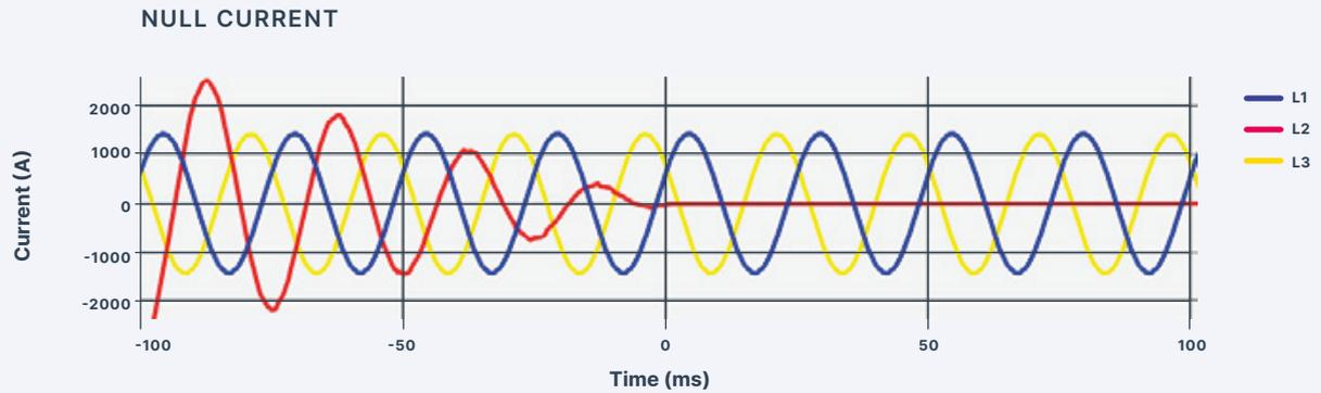
Figure 6 Null Current - Disconnection of the existing load, resulting in a null current in line L2.
